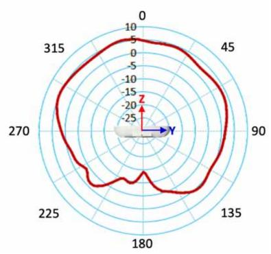
Figure 5 C9105AXI and C9105AXIT — BLE Antenna — Azimuth
