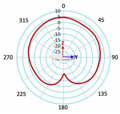
Figure 3 C9105AXI and C9105AXIT — Dual-band Antenna (5 GHz) — Azimuth
