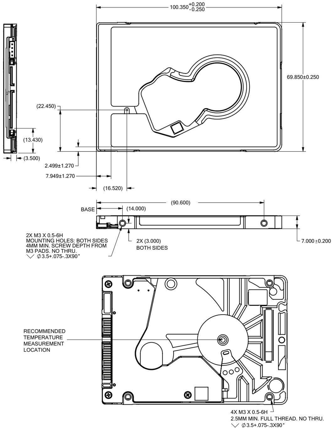
**Figure 5 Mounting Dimensions (for 2-disk models)**
